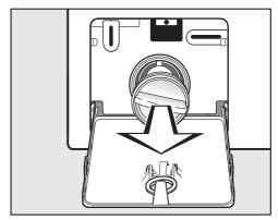
■ Remove the drain filter completely.
