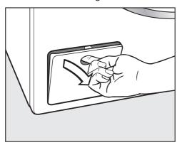
Open the drain pump flap.
