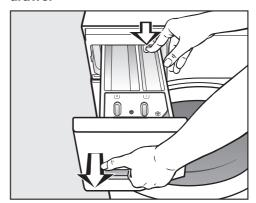
Pull out the detergent dispenser drawer until a resistance is felt. Press down the release button and at the same time pull the drawer right out of the machine.
