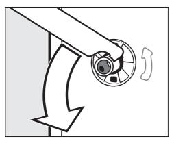
■ Using the wrench supplied, turn the left-hand shipping strut 90°, then
